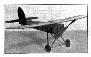
a pitch of 22 in., and therefore a pitch angle of 42 deg. Sheet brass, 1/16 in. thick, is used for the propeller bearing, and is shaped and bound to the fuselage as shown in the drawing. A plain bearing and propeller shaft is used as a mounting for the propeller. The rear rubber hook is of 1/16 in. steel rod, which is bent to shape, and fastened to the rear of the fuselage by binding and glueing as shown in the drawing. Ten feet of  $\frac{1}{8}$  in. flat rubber is used for the motive power.
