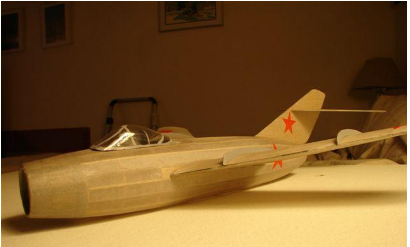
Mig-15 wing mount to flush sheeting
