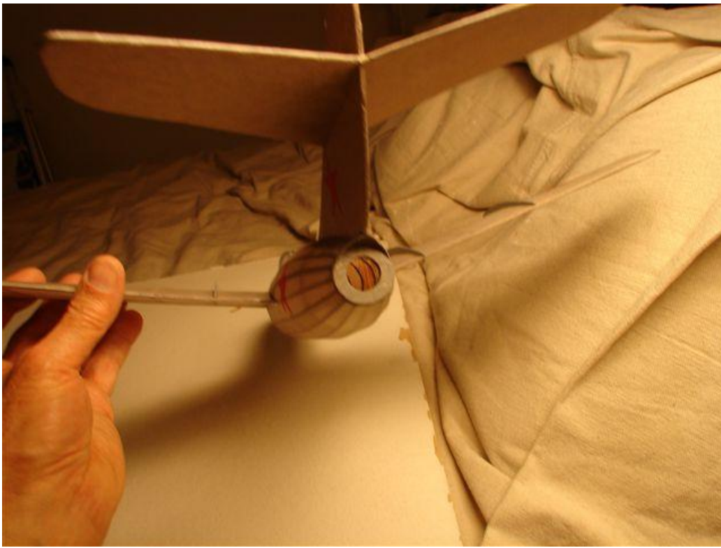
Mig-15 back end shows hole for motor, and formed fairing.
