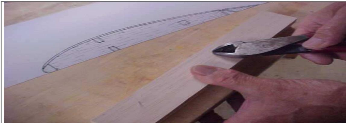
**A side cutter makes short work of trimming the pins as close as possible to the wood.**
