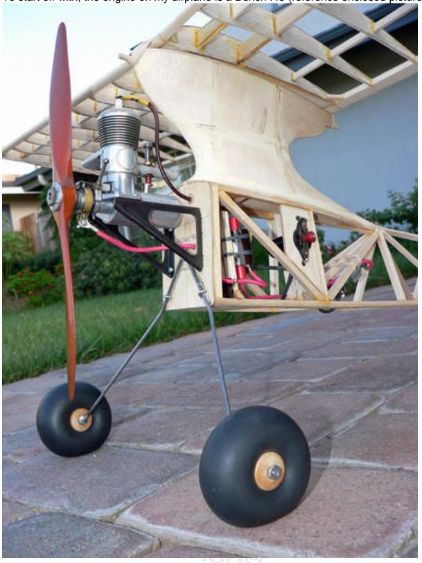
The engine mount is a K&B stamped steel two piece unit that I bought at a MECA swap meet. The wheels are off the shelf Trexler Airwheels. I think they are 2 1/2". These are currently in production and available through Penn Valley Hobby Center in Pennsylvania or on the internet.
