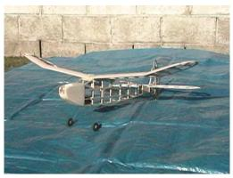
Finished aircraft flies with throttle, elevator and rudder. Cox TD .020 with throttle for power, Hitec Electron 6 receiver, three HS-55 servos and 110 mah battery. Covered with Coverite "Coverlite" fabric.
