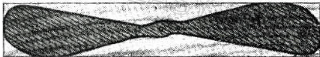
Fig. 18.—The propeller is carved out of a piece of satin walnut, and a hole bored in the centre to take the gear spindle.
