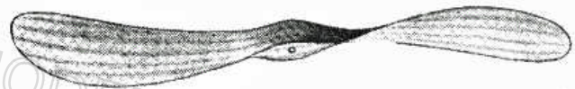
Fig. 19.—The finished propeller. The centre is kept thick, while the sides are shaped thin with a wood-rasp and glass-paper.
