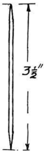
(Left) Fig. 7.—One of the five ribs used in the construction of the mainplane.
