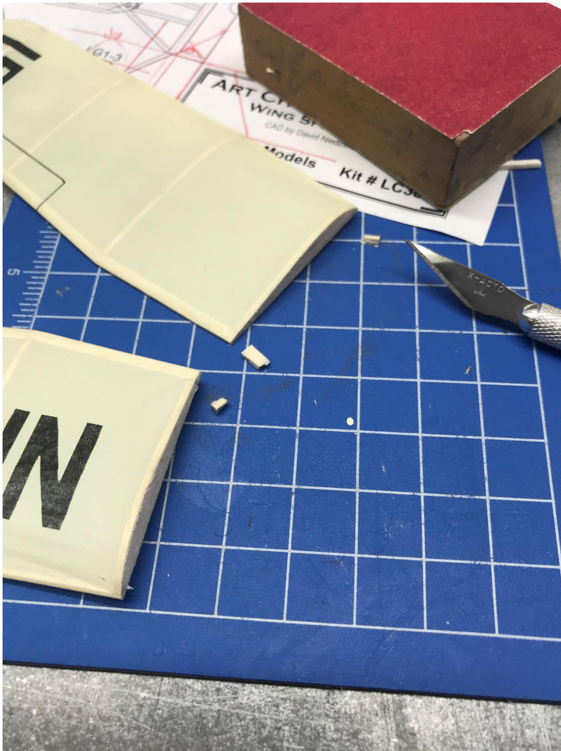
73. Since this is a butt joined wing, I trimmed the LE and TE flush with the outside of the root rib. Sanded to be sure flush.
