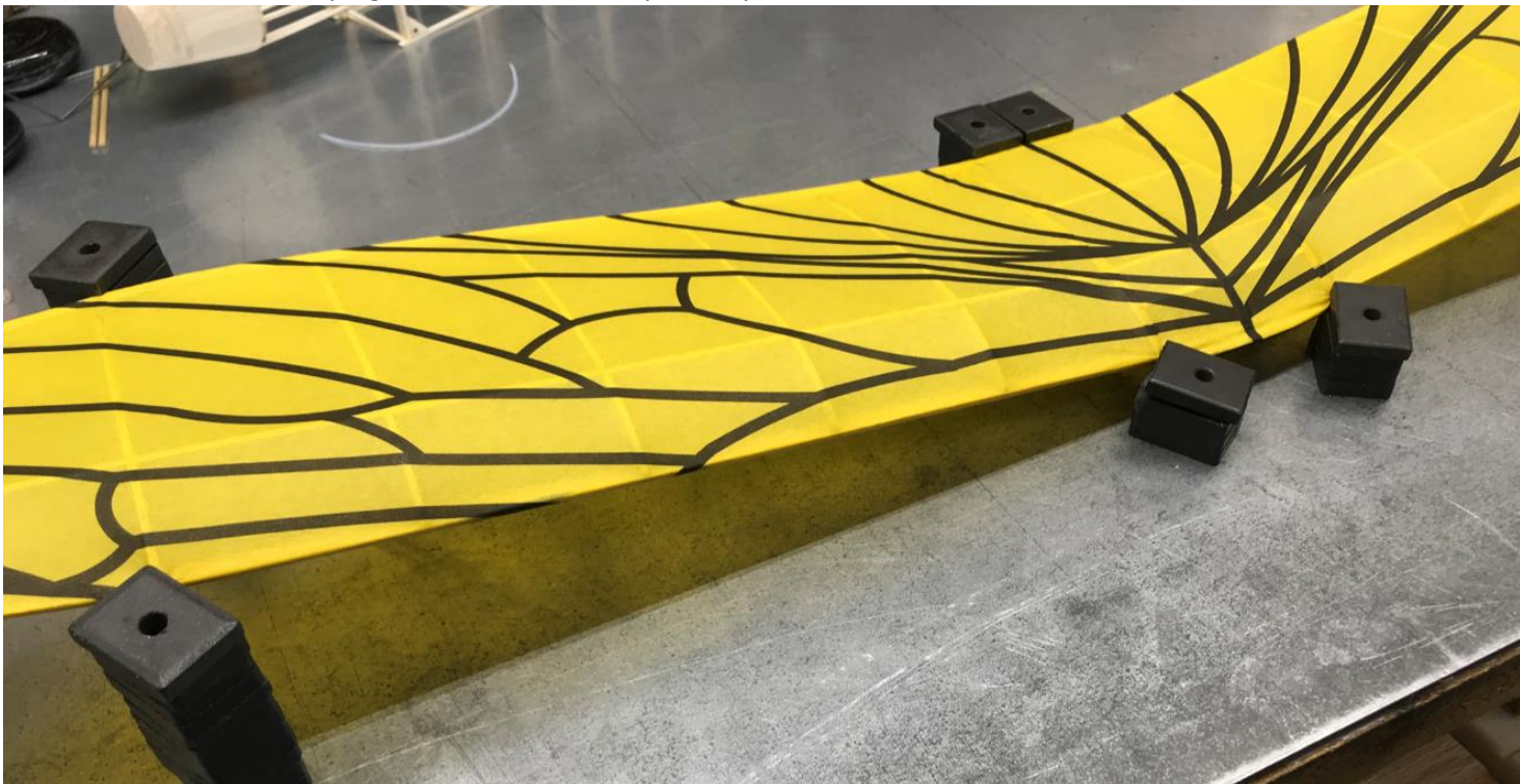
41. I actually elevate the wing on magnets when I'm clamping it down so that air can pass under and over it for even drying.
