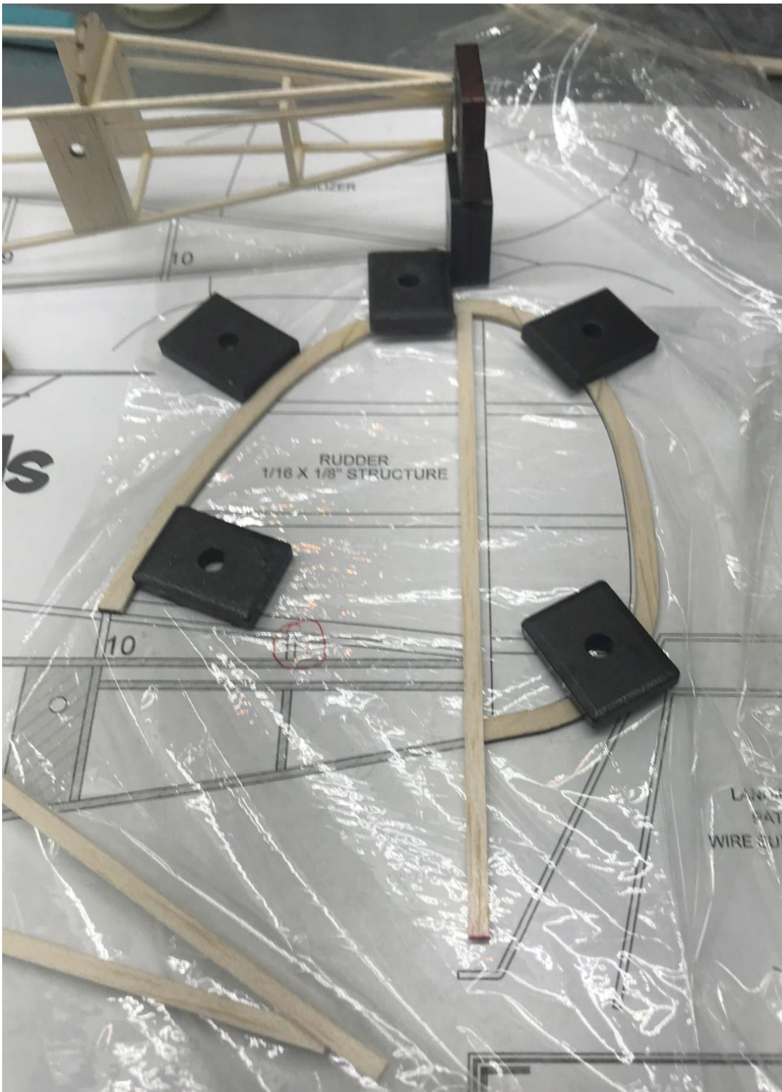
12. While the stab halves dry, I move on to the rudder which is assembled very similar to the stab.
