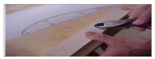
A side cutter makes short work of trimming the pins as close as possible to the wood.
