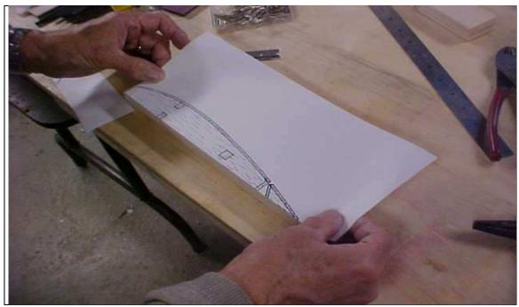
The back of the template has been sprayed and now it needs to be aligned to our balsa. The base of the balsa has been sanded even. We position the template to the base of our balsa and begin smoothing down.
