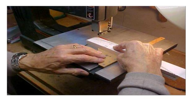
I use a square with my band saw to cut the front of the rib to 90 degrees or what ever is required. The band saw cut straight unlike a scroll saw. Use a metal cutting blade as it has more teeth and a smother cut is made in the soft balsa.
