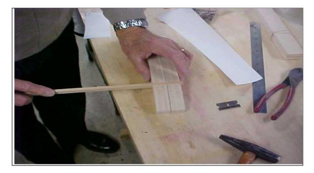
This is where we test fit our spar to the top and bottom of our prepared ribs. If necessary use a spar sanding tool to expand or deepen the slot.
