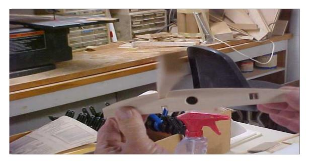
Spar is test fitted through all ten ribs top bottom. Note round hole which will be used for the wiring of the servo. Note the square hole. That was also test fitted with the spar for proper fit.
