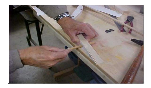
Use a small square piece of balsa and glue sand paper to two sides. Work the tool top to bottom and side to side to get a nice square hole. Don't over do it as you are going to test fit the main center spar that runs through all the ribs.
