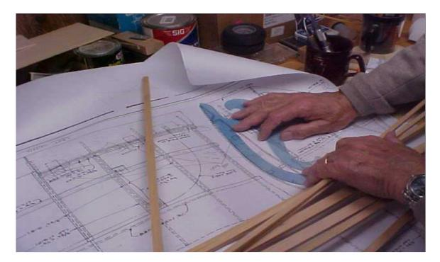
Using the French square. Use of the French curve is more time consuming than duplicating your plan. However if you want to make permanent templates from plywood the French square duplicates the original rib very close. This can be done by pinning down the plans over a piece of tracing paper and paper underneath the tracing paper.
