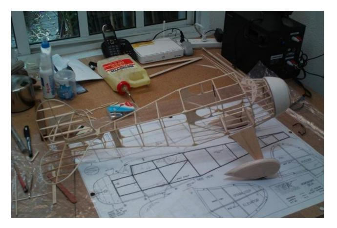
Here you can appreciate the profiled rudder and stab and the landing gear to absorb better the shock (well, I hope so haha!).
