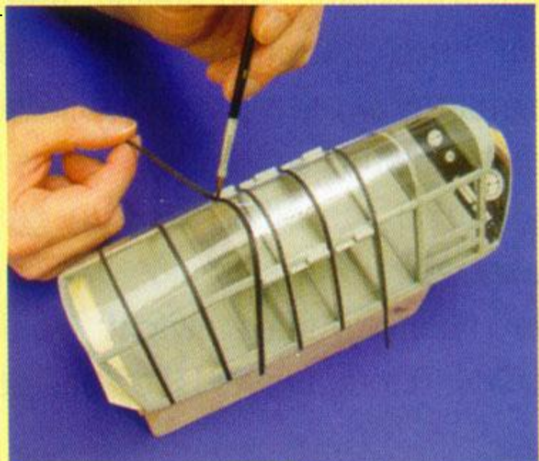
Strips of black tissue, glued on with dope imitate the cabin supports and make the glued joints invisible.
