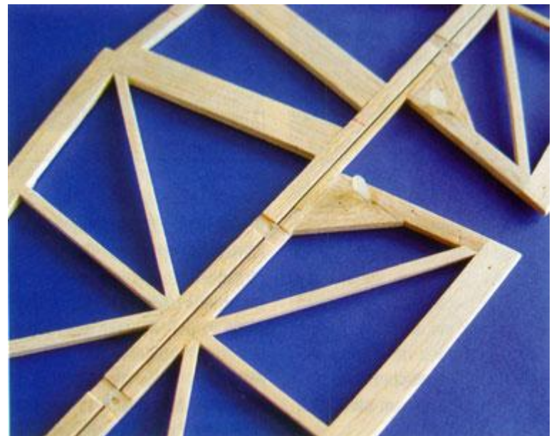
Narrow strips of material set into the upper surface of the spars serve as rudder flaps.
