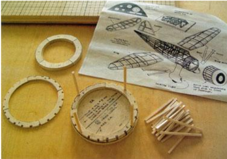
The motor cowling is made of ring-formers & balsa strips.
