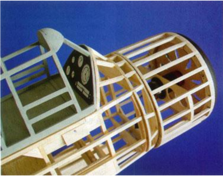
The motor cowling is glued to the fuselage, the motor is in the dummy star-motor, and a helping former placed in such a manner that it can be pulled from the inside out into the motor hood. Visible too are the connections of the cabin cowling.
