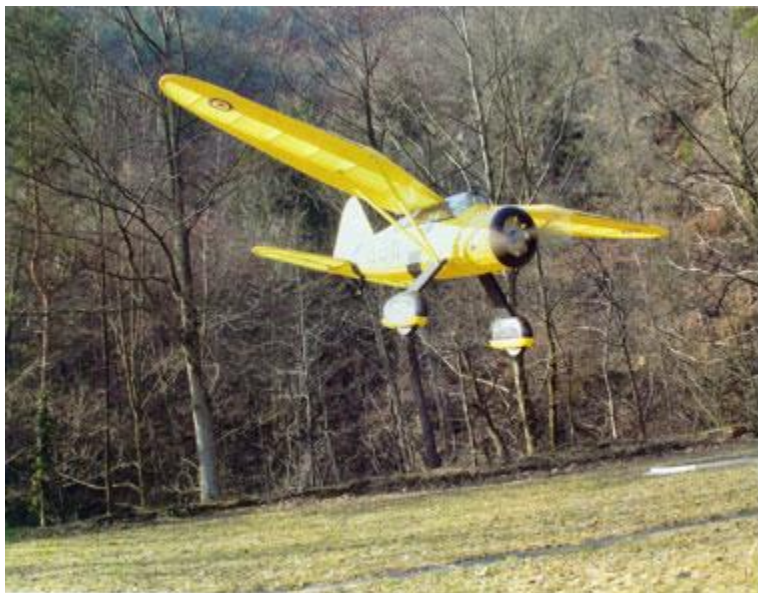
A light electric motor and 2 LiPo cells enable the Lysander to attain a pleasing duration of flight.
