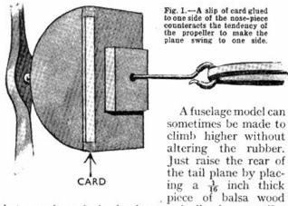
between it and the fuselage, and tilt the propeller forward by placing another similar piece between the top of the nose-piece and the fuselage (Fig. 3). Strap the nose-piece into place, or the packing will be shaken out by the vibration of the propeller. If the fuselage model is slow or low-powered, it may be necessary to fit extra rubber, in which case do not forget to move the wing back, and try flying with a few turns before you wind fully.
