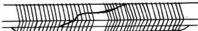
Fig. 6.—Even a broken wing spar is repairable by means of a splint and thread binding, as shown.
