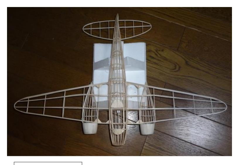
You can see just how much the plane has been lightened by removing much of the framework.
